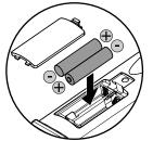
Make sure to match + and - on the batteries to the marks indicated in the battery compartment.
